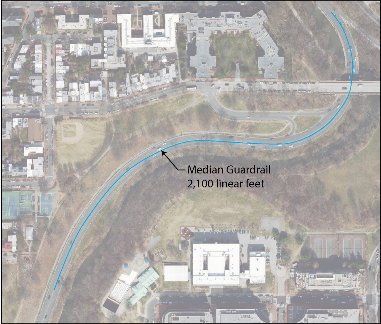
Figure 45: Conceptual Plan of RCPP at P Street, Median Installation and Exit Ramp Closure
